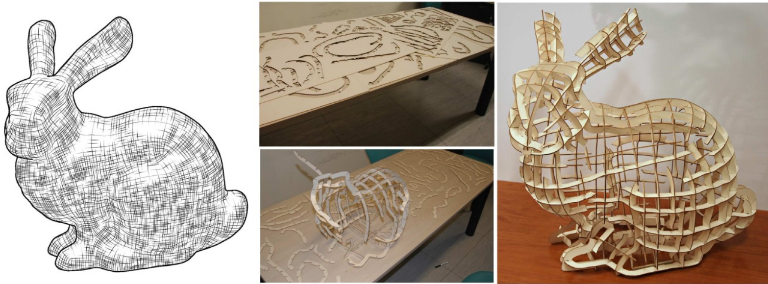
Fig. 1. Given a 3D shape with a smooth cross-field, we generate a set of planar slices that can be interlocked in a self supporting structure.
